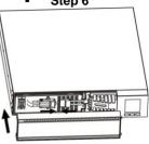
Remove the top cover of battery box and replace the inside batteries.
