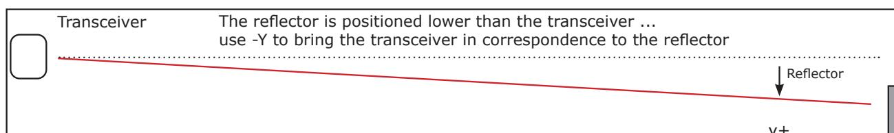
The BDH160 optical beam smoke detector can be moved on both the X and Y axes up to a maximum of 5 degrees by means of the **left (x-)**, **right (x+)**, and the **up (y+)** and **down (y-)** keys.
