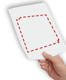
**Fire** – Slowly cover 70% of the reflector with a non-reflective card to simulate smoke that obscures the optical beam of the BDH160 detector. After 10 seconds the detector should detect fire status and the red light should start flashing.
