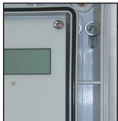
Use the screw holes on the outside of the rubber seals. Connect the control unit in accordance with the colours indicated on the terminal block. If this connection is not completed correctly, an ERROR message will be shown on the control-unit screen; this connection can be checked by reading the resistance between the black and grey terminals: a value of 110 Ohm is considered correct, while a value of 220 Ohm indicates an incorrect connection.
