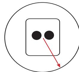
The field of view of the BDH160 has a radius of 50cm from the centre of the detector and must be free of obstacles.
