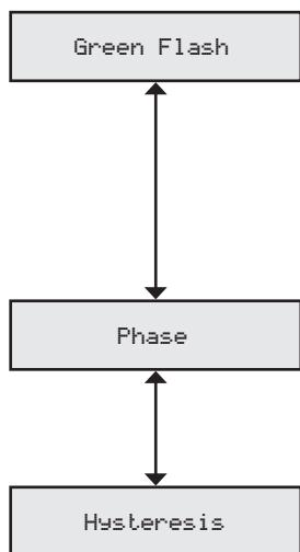
**Green Flashing Light on/off.** Using the **right** and **left** keys it is possible to **turn on** or **turn off** the green flashing light located on the transceiver and on the control unit. This is a useful way of finding the transmitter you are working on (press **enter** to return to the **settings** or the **down** key to switch to the **Phase** function).
