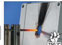
■ Burning behaviour: glow wire test in accordance with IEC 60695-2-11: 750 °C, flame-retardant, self-extinguishing
