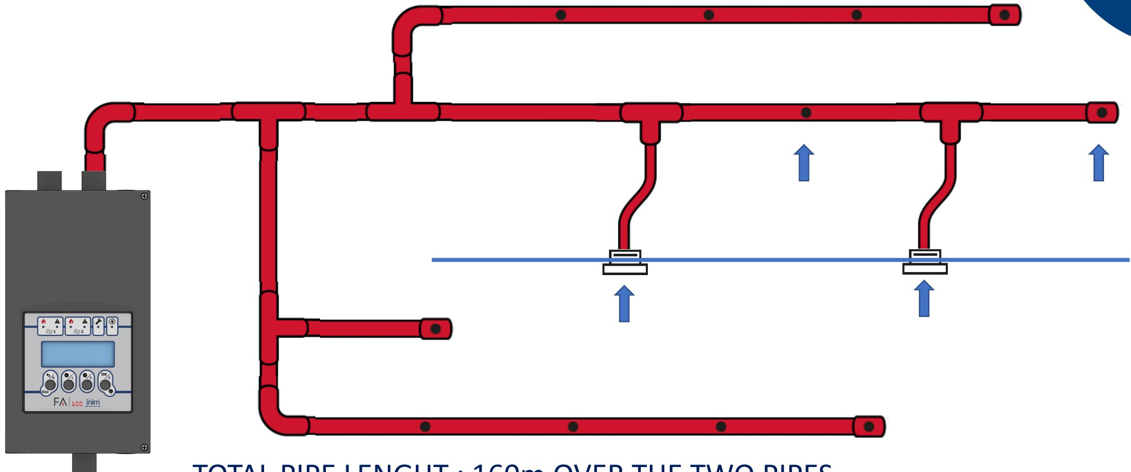
TOTAL PIPE LENGTH : 160m OVER THE TWO PIPES
