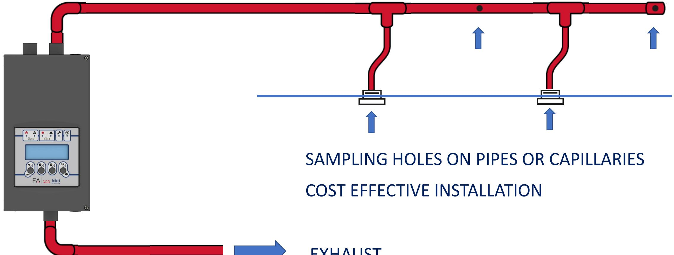
SAMPLING HOLES ON PIPES OR CAPILLARIES
