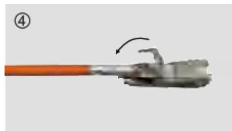
5. Fasten supplied cable tie to secure grounding contact.
