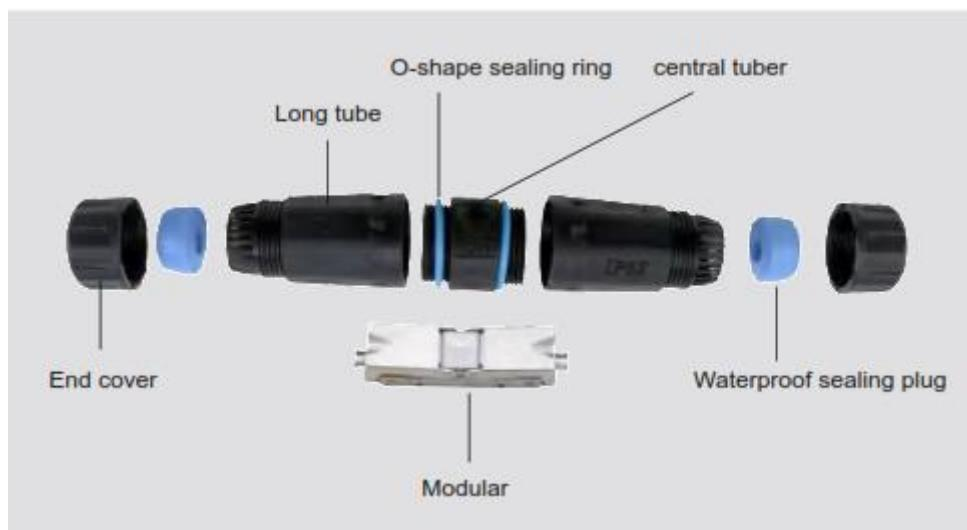
1. Pass one cable through the end cover, the long tube, and central tube in turn; pass the other cable through the end cover, long tube in turn.
