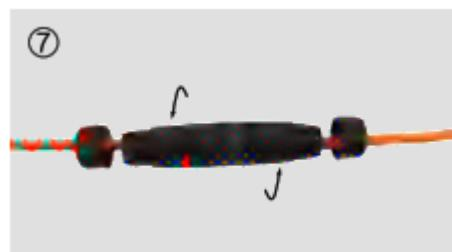
8. Lock the two waterproof plugs on the cable, then put them into the end of the long tube. Note: The plug is engraved with the word "waterproof" on one side outward.
