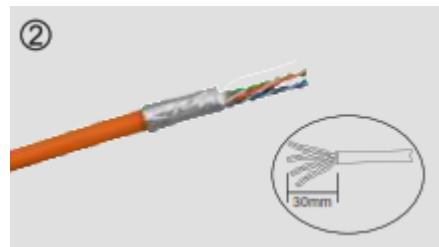
3. Fan out four twisted pairs, following the color coding label and allocate each conductor into proper slots on wiring cap. Trim the ends of conductors.
