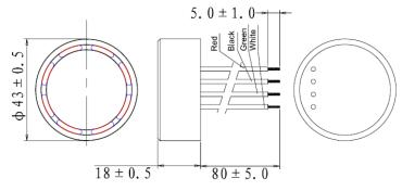
Dimensions : Millimetres Tolerance: ±0.5mm
