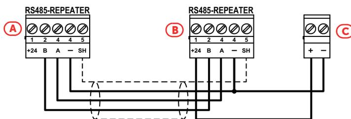
In this case the power to the repeaters [B] is not supplied by the control panel [A] but by an external power supply [C].
