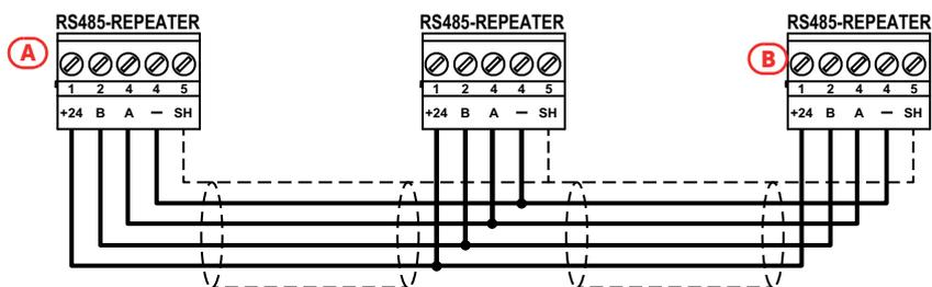
The jumper for the position on the BUS (paragraph 3.4 - [Q]) must be inserted in the EOL position EOL for the control panel [A] and for the end-of-line repeater [B].
