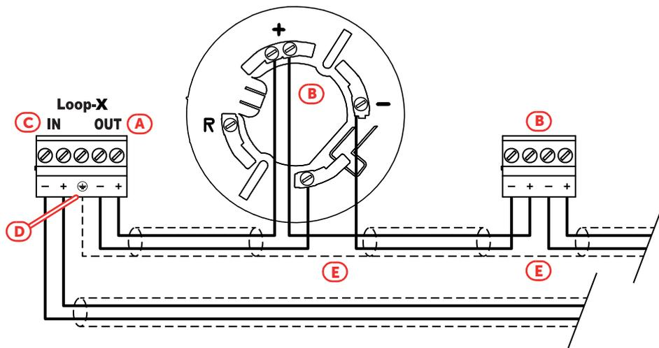
When connecting the loop devices it is not necessary to follow the input/output order indicated in the figure. Connect the cable shield only at the start of the loop (*(D)*), the shield can be connected to the terminal indicated in the figure or directly to the grounding bar). Take care to link the interrupted shields in correspondence with the device connections (*(E)*).
