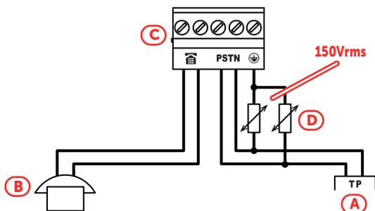
Connect the telephone line [A] to the PSTN terminals and telephone device or the internal phone line [B] to the terminals on the IFMDIAL module ([C], paragraph 3.15 - [E]).
