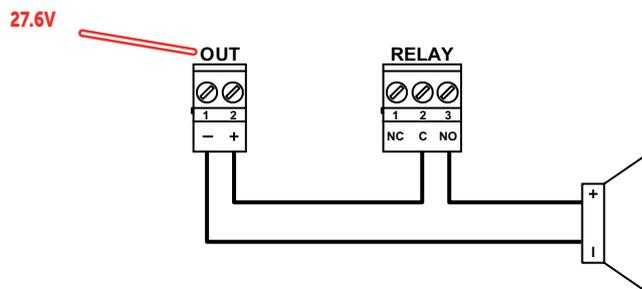
The OUT output illustrated in the diagram is used as a power source and is programmed as continuously active.
