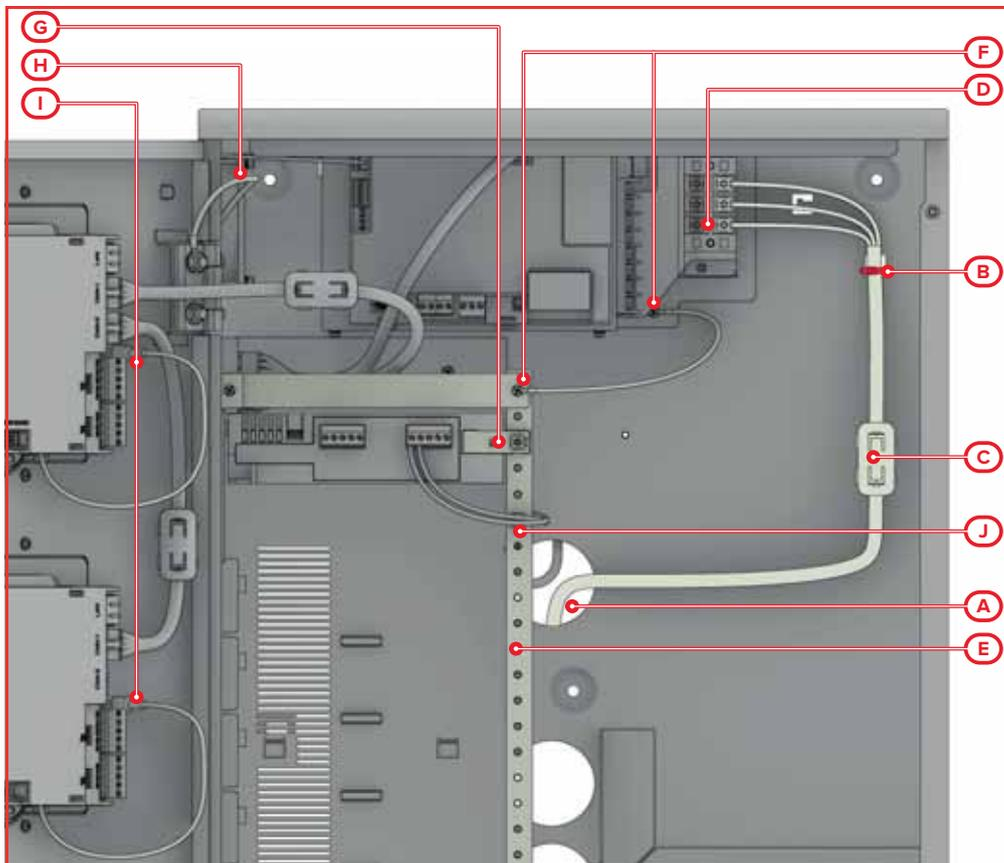
A dedicated input [A] must be provided for the mains power input terminal (230-115V~). The cable must be secured to the appropriate hooks by a plastic cable tie in order to avoid accidental dislodgement [B]. The cable must be protected by a ferrite (supplied) which must be affixed in the proximity of the terminals [C].
