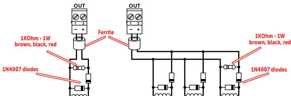
The polarities refer to the active status of the output, the polarities invert for stand-by status.
