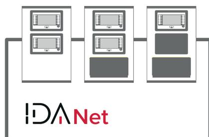
Through IDANet network-connection technology, Previdia Ultra control panels can be connected in a ring via a CAT5 ethernet cable (up to 100m) or optical fiber (by means of an appropriate SFP module according to the type of fiber used).
