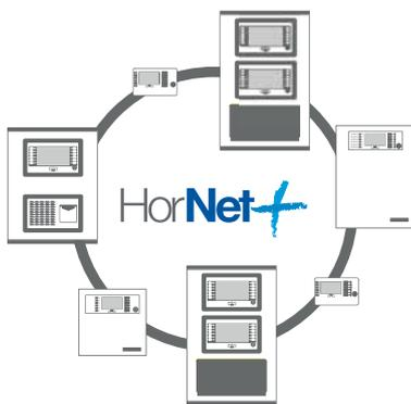
To increase the extension of the system with fire-fighting functions, it is possible to network several Previdia control panels (Ultravox, Vox, Ultra, Max or Compact up to a maximum of 48) in order to form a system of increased capacity (Hornet+ network).
