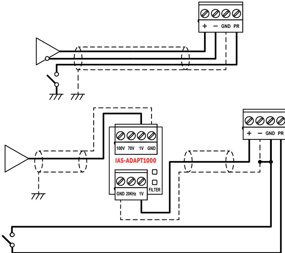
**Note:** *The priority request on AUX inputs can be detected on the audio signal level (option to be configured)*
