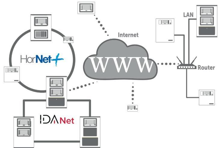
**Attention:** *The control panel that acts as a gateway for TCP-IP networking must include the FPMCPU module.*
