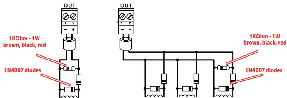
The polarities refer to the active status of the output, the polarities invert for stand-by status.
