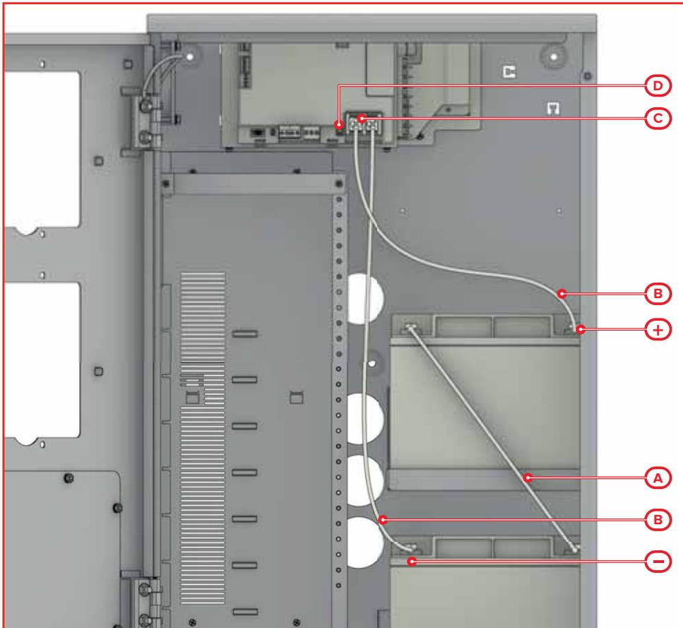
The batteries must be connected to the power-supply module by means of the supplied wires. They consist of two cables with connectors for the battery terminals and, for IFM24160 only, also a thermal probe (NTC) for temperature related charging voltage compensation.
