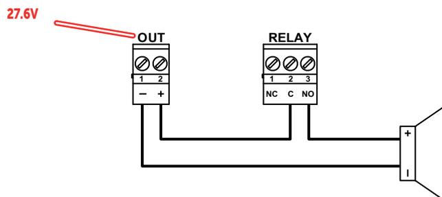
The OUT output illustrated in the diagram is used as a power source and is programmed as continuously active. The illustrated connection does not supervise the cable and does not signal connection faults.
