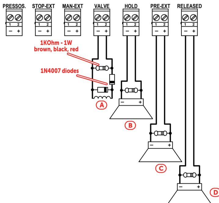
**4.20 J and E type relay output wiring (EN54)**
