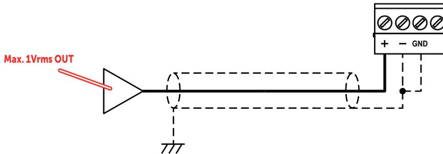
To avoid humming caused by ground loops, we recommend using the IAS-ADAPT1000 decoupling module.
