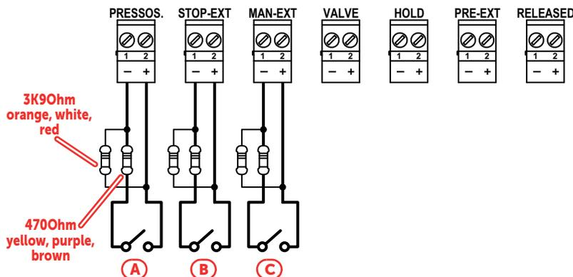
**Connection of output channels**
