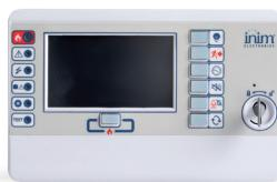
PREVIDIA-C-REP with customizable 4.3" touchscreen LCD, buttons for basic functions and status LEDs. Connects to the HORNET+ network (dual RS485 connection) or via ETHERNET TCP-IP network. It provides detailed information about the entire network. Internal buzzer. Level 2 via key or code.
