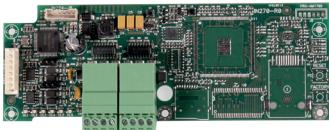
PREVIDIA-C-COM provides two RS232 ports and two RS485 ports for the connection of remote communicators, using the protocols available in the table.
