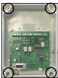
Picture 2 - Wall fixing screw holes, their distances from each other and the maximum allowed screw diameter
