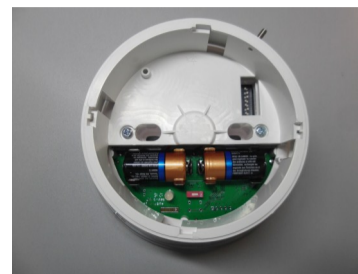
Picture 6 - primary and secondary batteries inserted
