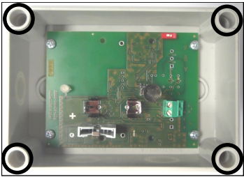
Picture 3 - Wall fixing screw entry points
