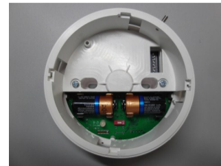
Picture 6 - primary and secondary batteries inserted
