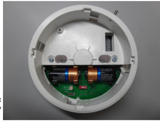
Picture 2 - wireless base sounder top view
